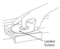
To retract the drawer back into the player after loading a disc, press the **Open/Close** button **2**. When the drawer is closed the display will indicate the total number of tracks on the disc and the total running time of the disc.
